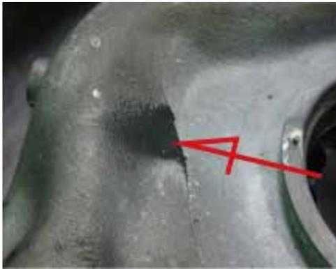
Crack of the housing
