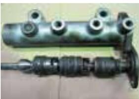
Deterioration of air cylinder (Infiltration of water/oil)
