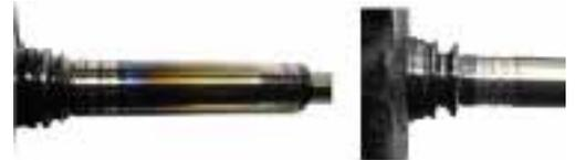
Diluted engine oil (Excessive worn for bearing)
