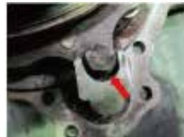
crank link of VG nozzle is worn
