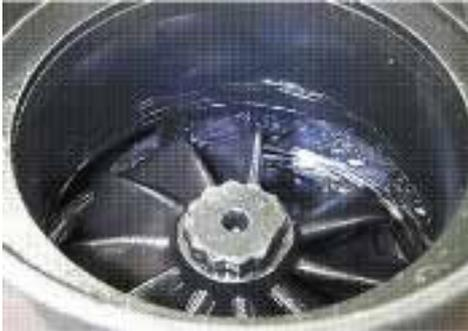
The reason for turbine wheel blade damage is high-cycle fatigue.
