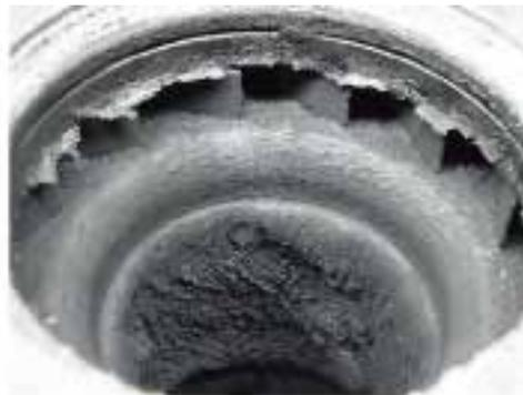
Accumulation of carbon on VG nozzle
