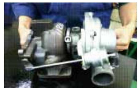
Do not rotate the rotor opposite way. It may cause damage to thrust bearing.
