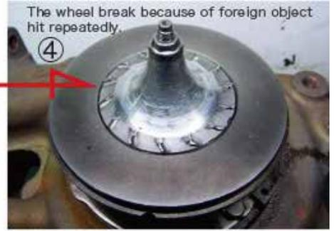
If the foreign object is big like nut, it cannot go through the narrow difuser passage of compressor housing. It also cannot go through the fin of the intercooler. It is difficult to go through the foreign object which may cause the damage to engine.
