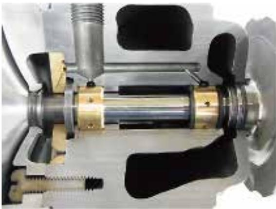
A lot of oil suction from breather , the oil in intercooler goes to engine and caused unusual combustion. **It may break by engine overrun.**
