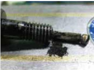
Carbon sludge can block union bolt
