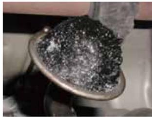
Sludge in centre housing oil inlet orifice.
