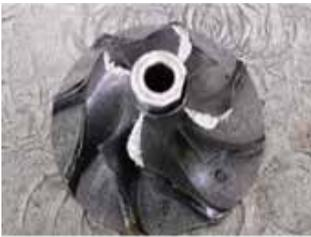
Foreign object damage on compressor wheel
